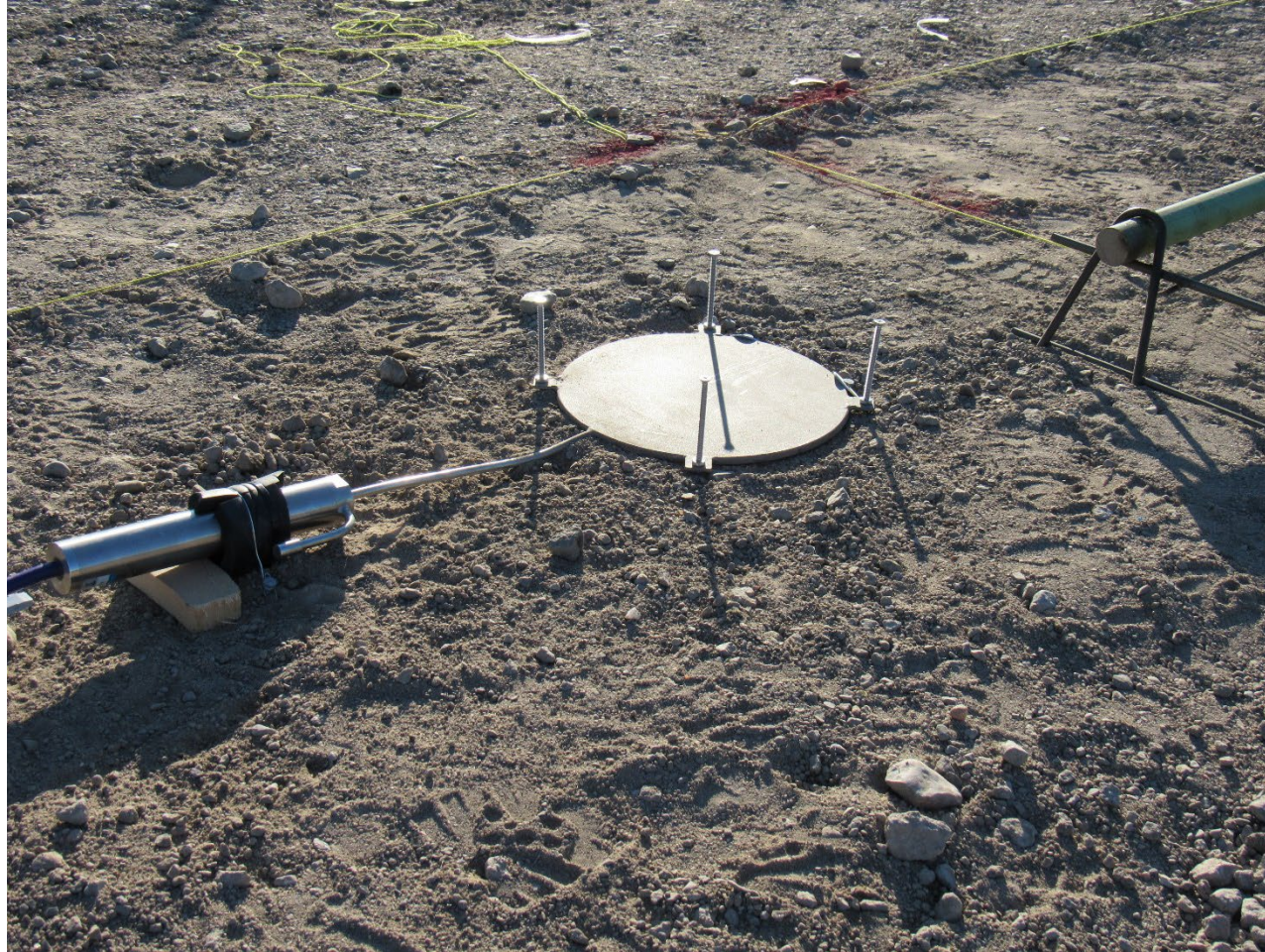
Pressure plate attaches to bottom of slab
