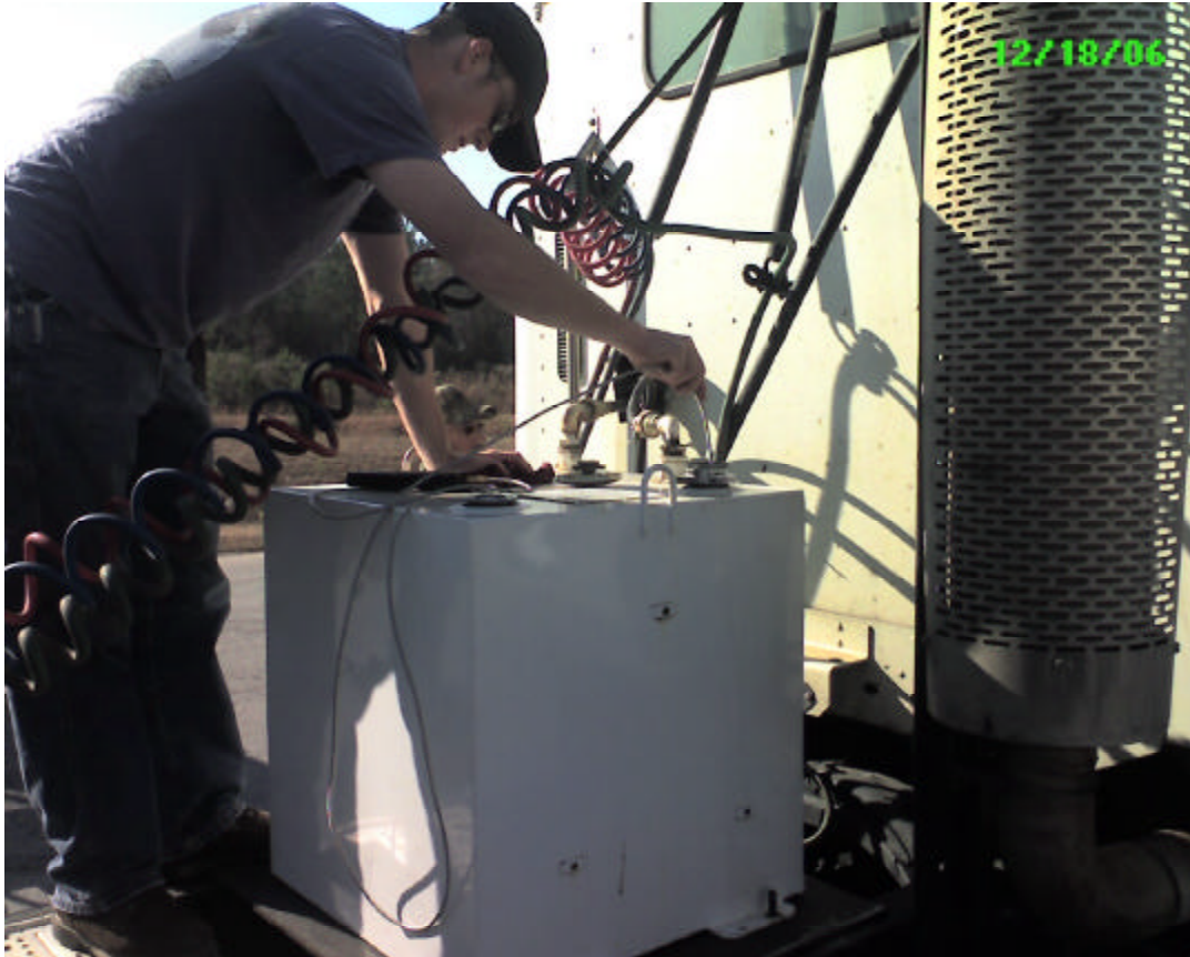
Figure 8 – Checking Temperature of Fuel in Portable Tank Between Test Runs
