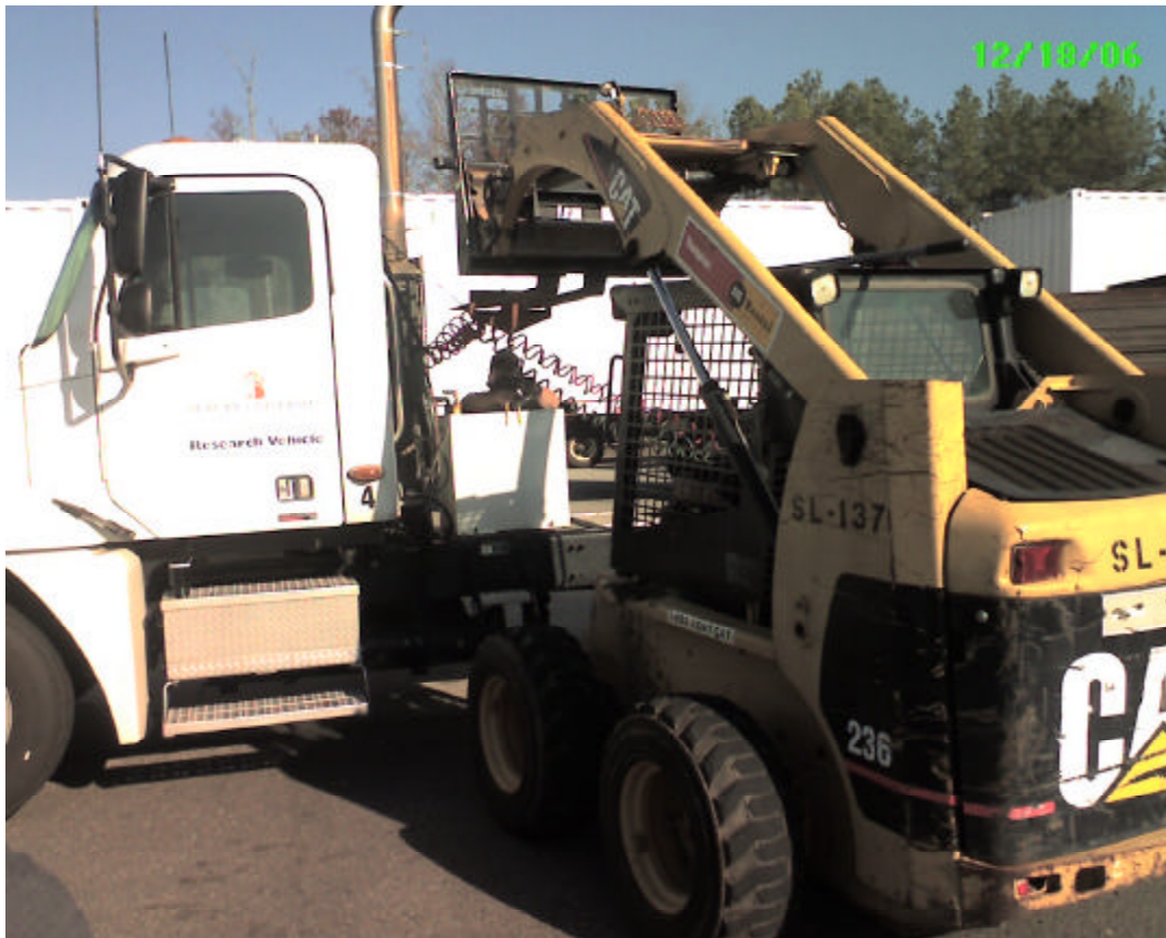
Figure 6 – Removing Portable Tank for Fuel Weight Determination
