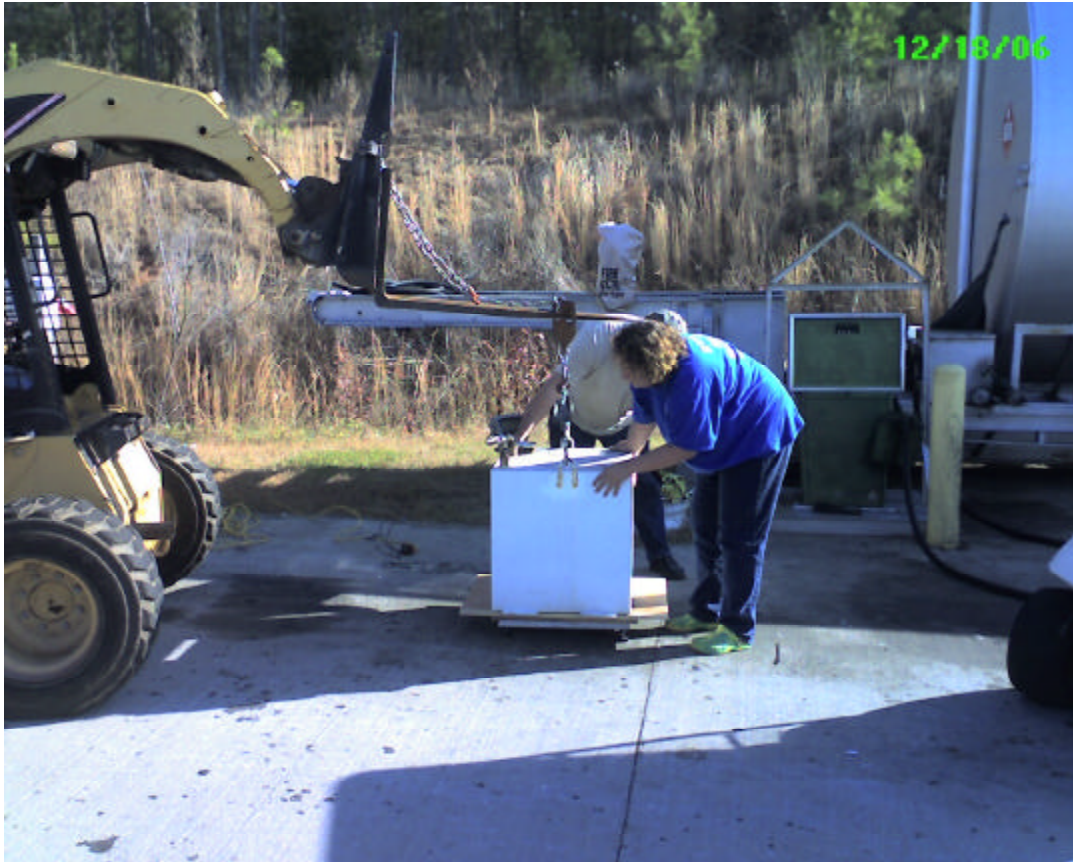
Figure 7 – Weighing Portable Tank to Within a Tenth of a Pound
